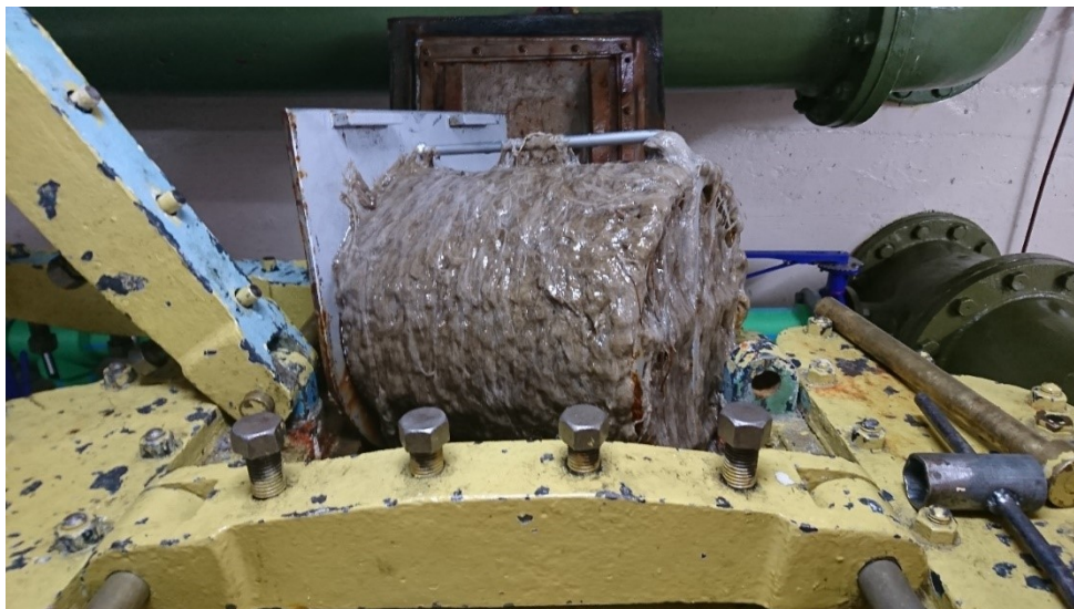
Fig. 3: Lindavia mucus at Lake Tekapo power station.
